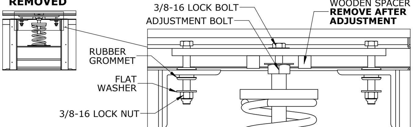
ii) Loosen two (2) 3/8-16" lock nuts located on either side of main spring until there is approximately 1/4"-3/8" space between flat washer and bottom of rubber grommet.
